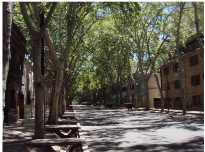
Figure 7. Street trees in low rainfall Mendoza, Argentina, are irrigated with water supplied by ancient gravity fed channel systems
